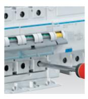
The RCD Add on block is equipped with locating pins which helps to secure the tightening of the bottom terminals to the circuit breaker. The cover cannot be closed if the terminals are not tightened correctly
