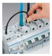
The connection of auxiliaries becomes easy, thanks to the new "Fast on" connection terminals provided on the to and bottom of the MCBs. This provided a quick and easy solution to feed auxiliaries such as shunt trip coil, UV release etc.
