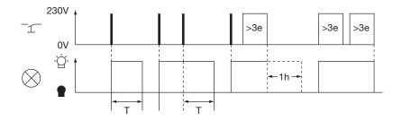
4. Double delay + Pre-warning mode: Press a push button briefly to switch ON the light. After an adjustable time "T", the light will switch OFF automatically. If you press the push button for more than 3 seconds, a time lag of one hour will start. A signal (blink) appears before the end of the lighting period.
