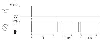
3. Double delay mode: Press a push button to switch ON the light. After an adjustable time "T", the light will switch OFF automatically. If you press the push button for more than 3 seconds, a time lag of one hour will start.
